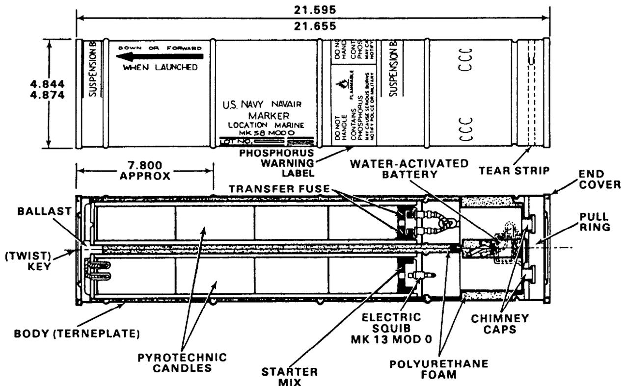
Figure 6-5.—The Mk 58 Mod 0 marine location marker.
