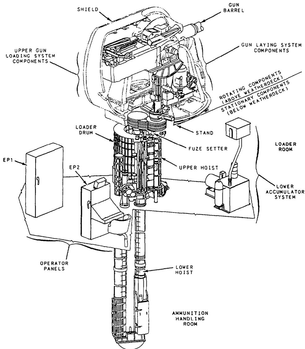
Figure 6-16.—The 5"/54 Mk 45 Mod 0, general arrangement.
