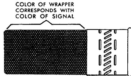
Figure 6-8.—The Mk 2 marine illumination signal.
