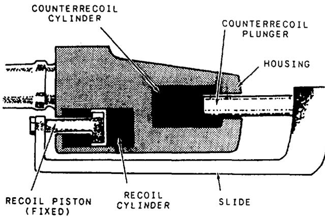
Figure 6-13.—A basic recoil and counterrecoil system.
