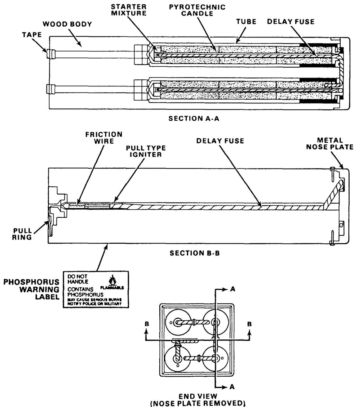
Figure 6-7.—The Mk 6 Mod 3 marine location marker.
