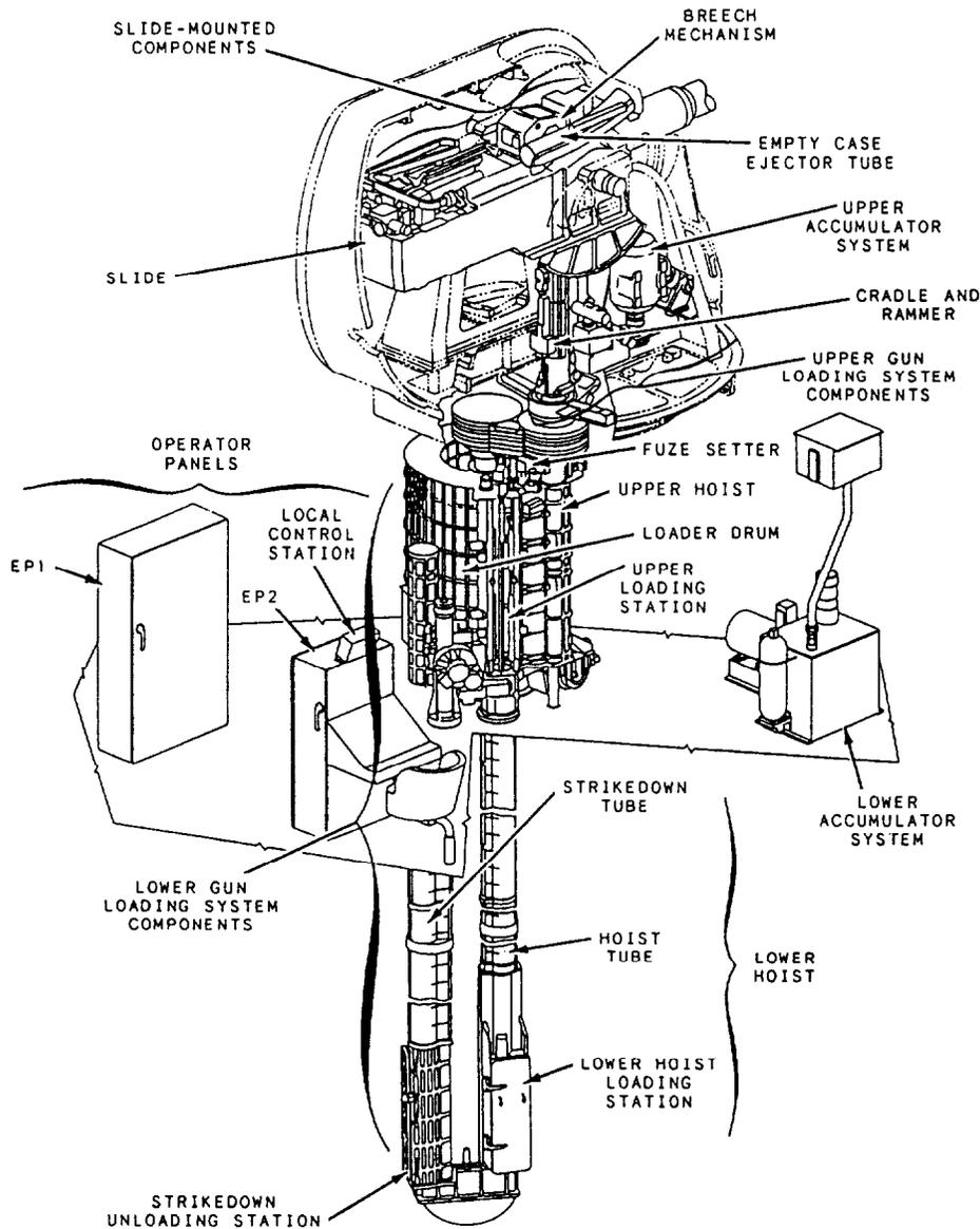
Figure 6-17.—The 5"/54 Mk 45 gun loading system, major components.
