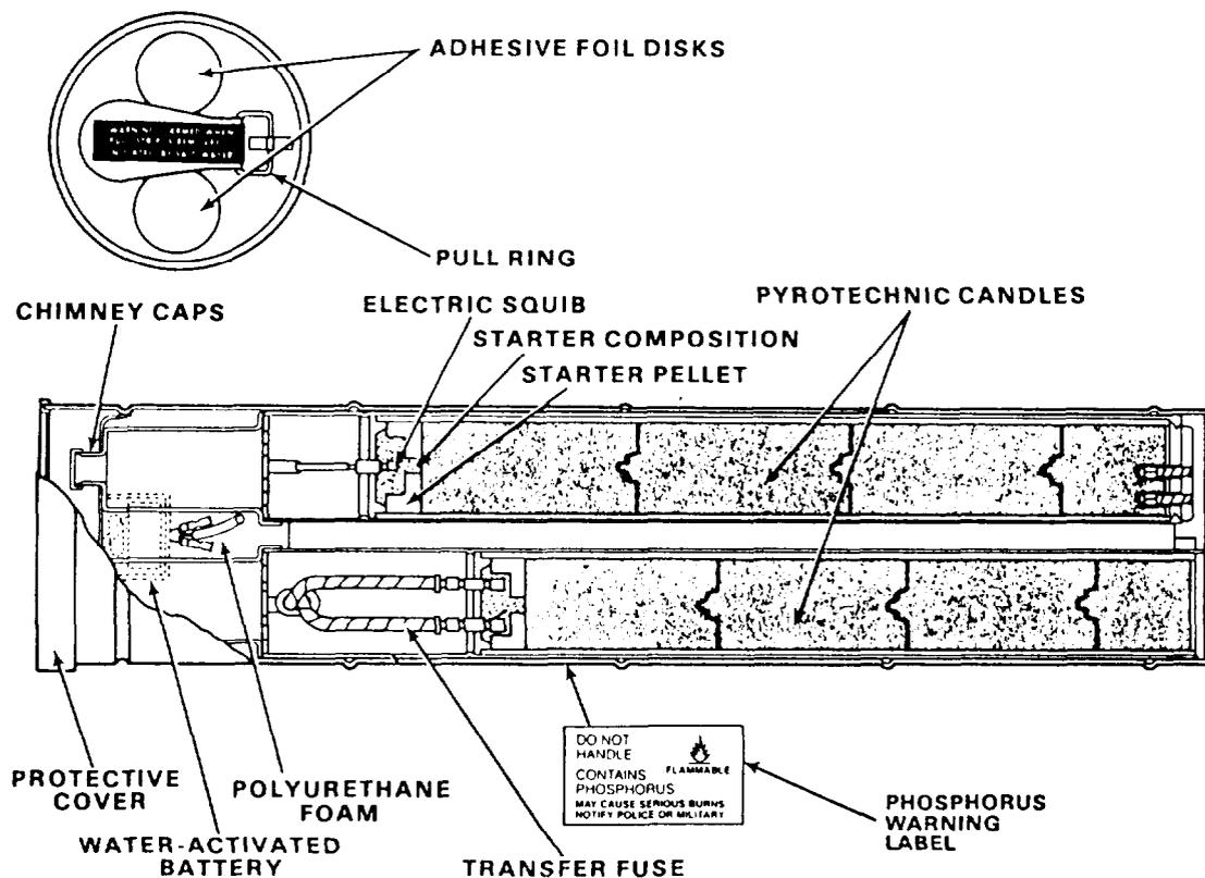
Figure 6-6.—The Mk 58 Mod 1 marine location marker.
