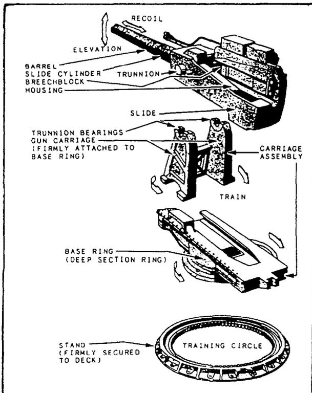
Figure 6-10.—Gun-positioning equipment.
