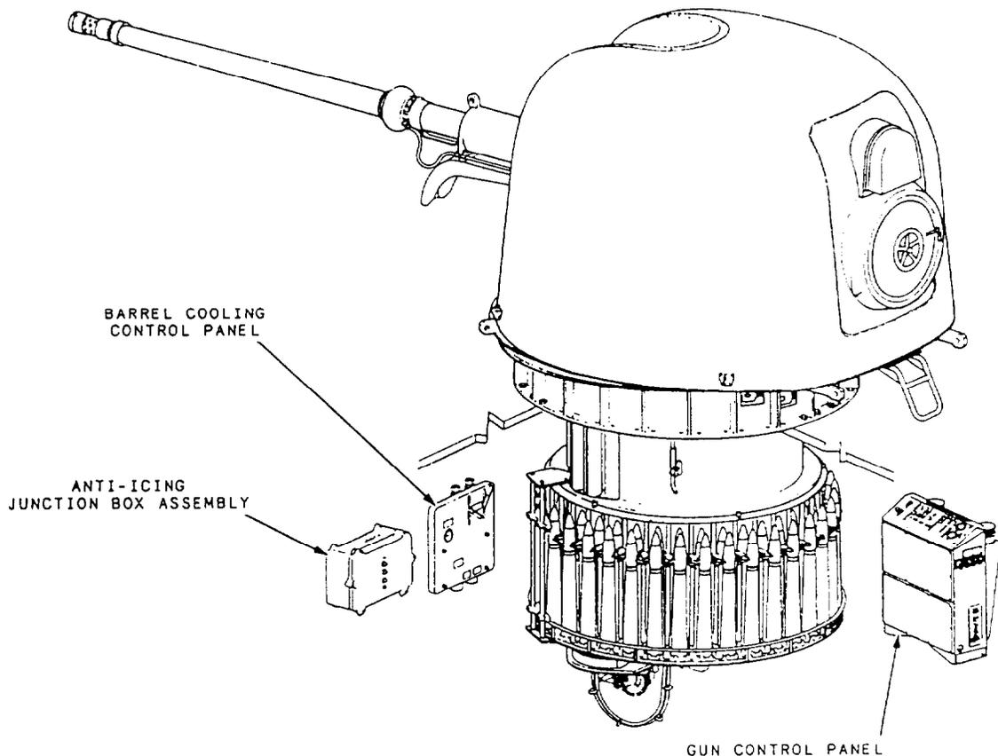
Figure 6-18.—The Mk 75 gun system, general configuration.
