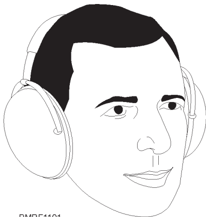
Figure 11-1.—Circumaural (Mickey Mouse) type of ear protector.
