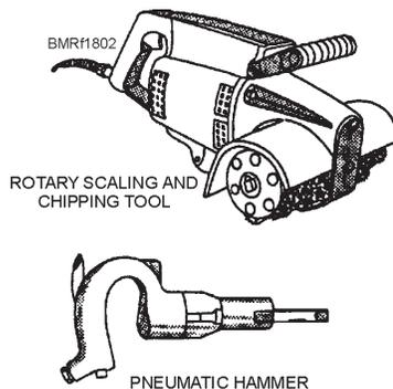
Figure 18-2.—Power scaling tools.
